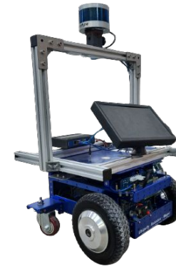
RAMP-Bot mounted with velodyne LIDAR and display monitor to visualize SLAM
